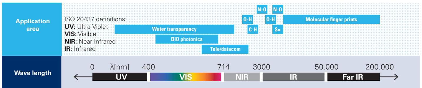
Figure 3 Wavelength of operation for applications<sup>1)</sup>
