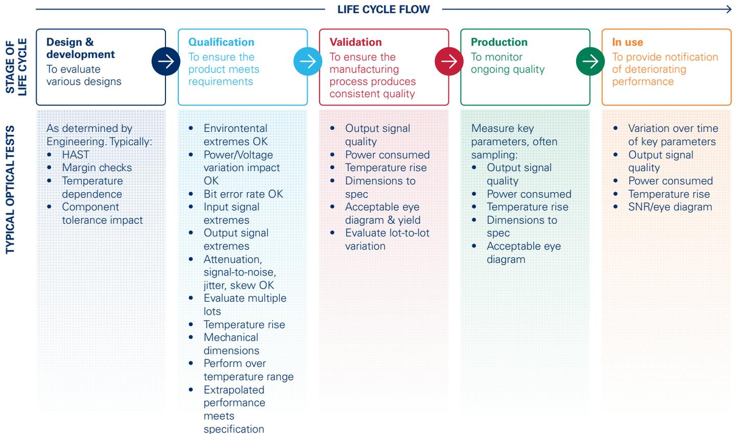
Figure 16 Test needs during an optical product life cycle<sup>14)</sup>
