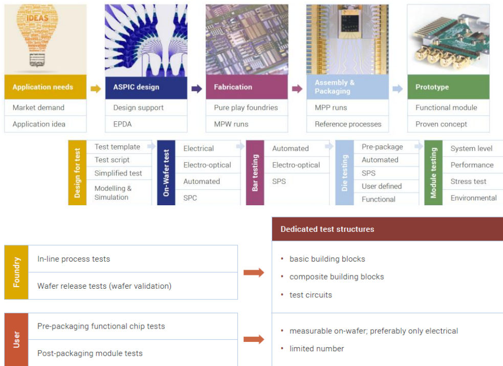
Figure 2: Testing across value/supply chain of Application Specific Photonic Integrated Circuits. (source: JePPIX roadmap 2018)
