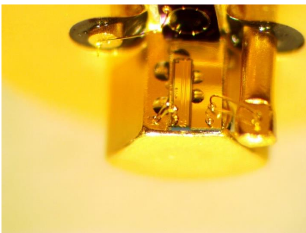
Figure 6: TO-56 style Laser assembly (Source: Voyant Photonics)
